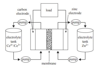
The following standard reduction half-cell reactions occur in the zinc-cerium cell.
